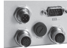
M12 railway power input and two Gigabit LAN connectors
