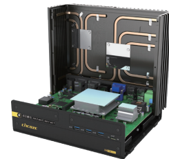
Independent cooling for CPU & GPU
