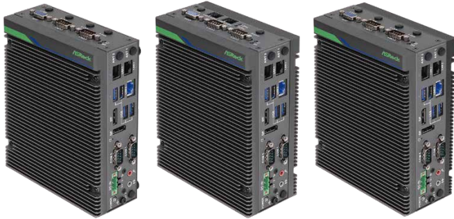
iEP-7020E-010 Series (Basic SKU) iEP-7020E-011 Series (PoE SKU) iEP-7020E-013 Series (5G SKU) iEP-7020E-012 Series (5LAN-Wifi SKU) iEP-7020E-013 Series (5LAN-5G SKU)
