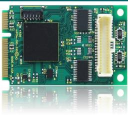
from the card. The digital I/O is compatible with 8255 PPI chips making it easy to program. This allows for simple and trouble-free migration from other ACCES PCI and PCI Express digital I/O cards, but also provides for advanced features enabled by the onboard FPGA logic.
