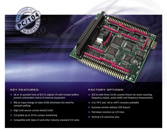
The 104-DIO-48S and 104-DIO-24S provide a total of 48 or 24 lines of digital I/O with counter/timer for PC/104-based data acquisition. This low-cost, high-performance, reliable board features Change of State (COS) detection on user-selected ports, allowing the board to generate an interrupt port by port. Since one READ determines the data, there is no need for constant polling, which greatly reduces processor overhead and allows applications to run more smoothly.
