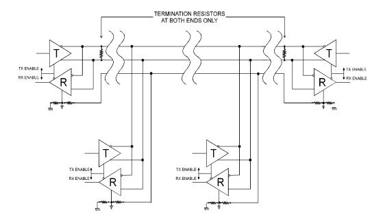
Figure A-1: Typical RS485 Two-Wire Multidrop Network
