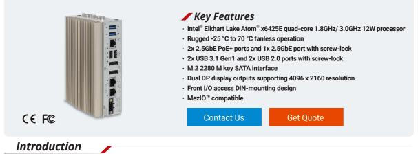
POC-400 is an ultra-compact fanless embedded computer for industrial applications. It utilizes the latest Intel<sup>®</sup> Elkhart Lake platform Atom<sup>®</sup> x6425E 4-core CPU that can deliver 1.7x CPU and 2x GPU performance improvement, compared to the previous generation.
