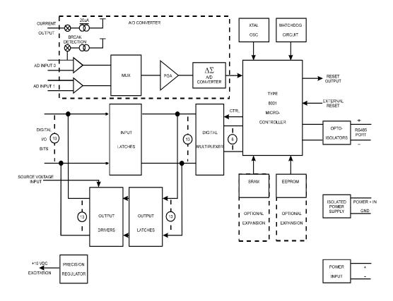
The built-in watchdog timer resets the pod if, for some unexpected reason, the microcontroller "hangs up" or the power supply voltage drops below 4.75 VDC. Data collected by the pod can be stored in local RAM and accessed later through the computer's serial port. This allows the pod to operate in a stand-alone pod mode.
