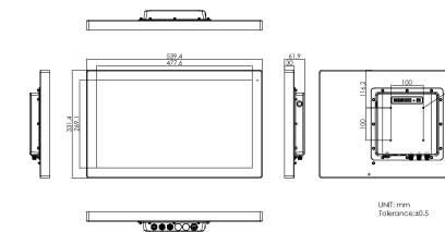
21.5" FHD IP66/IP69K stainless steel display, VGA/HDMI input, OSD on the rear side, projected capacitive touch, 9~36V DC power input with Adapter 21.5" FHD IP66/IP69K stainless steel display, VGA/HDMI input, OSD on the rear PhanTAM-121APH side, projected capacitive touch, 9~36V DC power input with Adapter, 1,000 nits LCD
