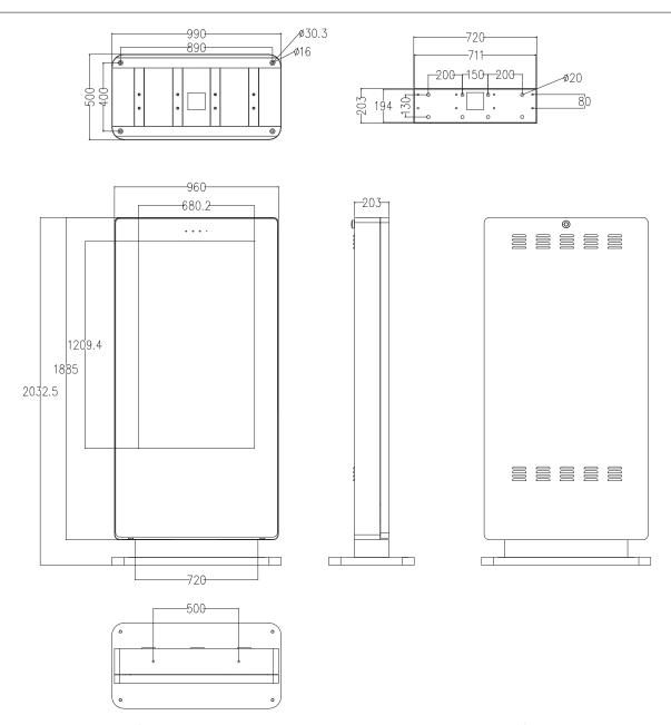
Note: The  $\varnothing 30$  holes are for access, we recommend using M10 anchor bolts that will fit into the  $\varnothing 16$  holes.
