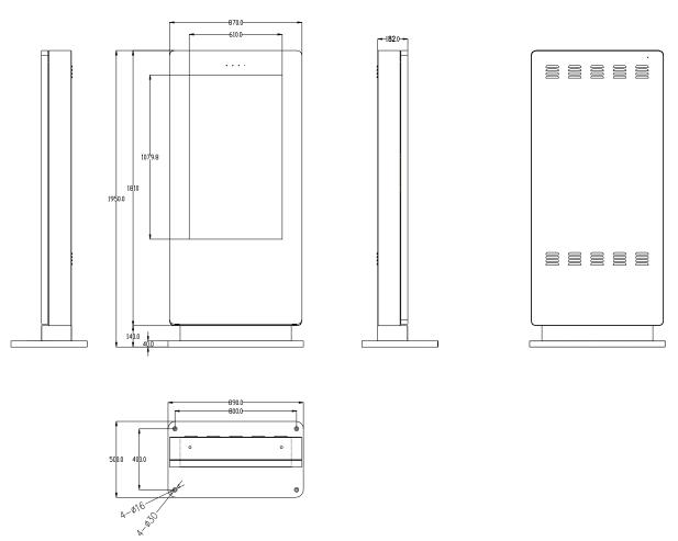
Note: The  $\varnothing 30$  holes are for access, we recommend using M10 anchor bolts that will fit into the  $\varnothing 16$  holes.
