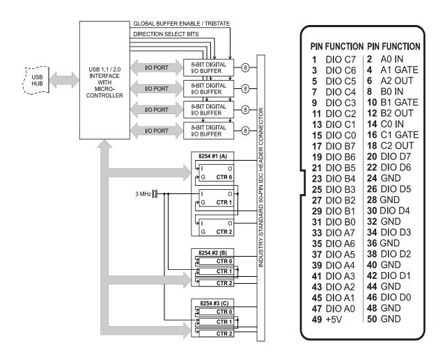
Table 1: Block Diagram and 50-Pin Connector Pin Assignments
