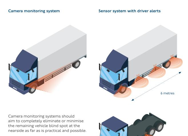
It is recommended that sensors on rigid vehicles and articulated tractor units have coverage six metres down the nearside or one metre from the rear of the vehicle (or tractor unit), whichever is smaller.
