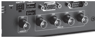
1 x AUDIO-IN + 4 x VIDEO-IN BNC connector for DVR surveillance system
