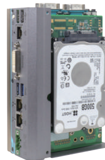
▲ POC-300 with MeziO™ - R11 and 2.5" HDD
