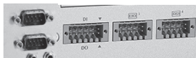
Isolated RS-232/422/485 ports (Optional DIO and 2 x COM module) (Optional CANbus / COM port)
